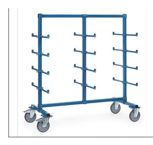
Modular system: Frame made of sturdy square tube. Cross beams, posts and bars connected with solid screwed joints. Carrier spars made of tubular steel Ø 27 mm with screwed joints. With 24 carrier spars on both sides (12 per side) with anti skidding device. Carrying capacity per level 120 kg (60 kg per side). Powder coated blue RAL 5007. 2 swivel and 2 fixed-wheel castors, TPE tyres, hubs with groove ball bearing. Swivel castors with wheel locks, according to EN 1757-3.
