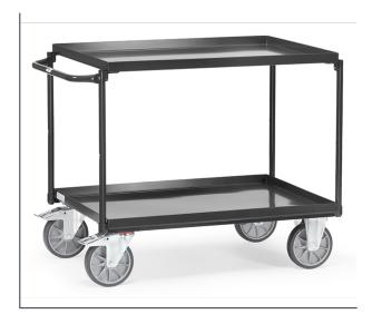
Modular system: Steel construction, welded. Tubular steel hoop and steel plate trays screwed. Trays oil-tight, rim 40 mm high, powder coated anthracite grey RAL 7016. 2 swivel and 2 fixed-wheel castors, TPE tyres, hubs with groove ball bearing. Swivel castors with wheel locks, according to the European Standard EN 1757-3 (safety of platform trolleys). Capacity of upper shelf 200 kg.
