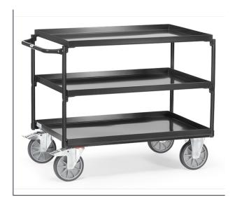
Modular system: Steel construction, welded. Tubular steel hoop and steel plate trays screwed. Trays oil-tight, rim 40 mm high, powder coated anthracite grey RAL 7016. 2 swivel and 2 fixed-wheel castors, TPE tyres, hubs with groove ball bearing. Swivel castors with wheel locks, according to the European Standard EN 1757-3 (safety of platform trolleys). Capacity of upper and middle shelf 200 kg.
