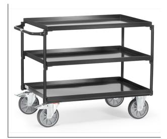
Modular system: Steel construction, welded. Tubular steel hoop and steel plate trays screwed. Trays oil-tight, rim 40 mm high, powder coated anthracite grey RAL 7016. 2 swivel and 2 fixed-wheel castors, TPE tyres, hubs with groove ball bearing. Swivel castors with wheel locks, according to the European Standard EN 1757-3 (safety of platform trolleys). Capacity of upper and middle shelf 200 kg.
