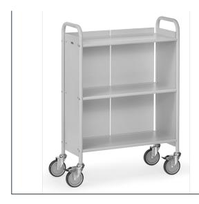
Modular system: bolted, tubular steel construction, powder coated light grey RAL 7035. Shelves and panels made of derived material timber board, pale grey. With longitudinal wall (back wall). 4 swivel castors with TPE tyres, hubs with roller bearings. 2 swivel castors with wheel locks, according to the European Standard EN 1757-3 (safety of platform trolleys). Flat packed for easy self assembly.
