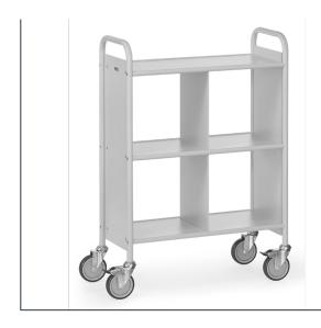
Modular system: bolted, tubular steel construction, powder coated light grey RAL 7035. Shelves and panels made of derived material timber board, pale grey. With separating plate. 4 swivel castors with TPE tyres, hubs with roller bearings. 2 swivel castors with wheel locks, according to the European Standard EN 1757-3 (safety of platform trolleys). Flat packed for easy self assembly.
