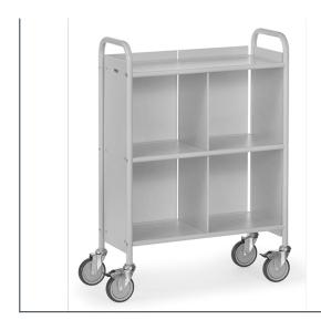
Modular system: bolted, tubular steel construction, powder coated light grey RAL 7035. Shelves and panels made of derived material timber board, pale grey. With separating plate and longitudinal wall (back wall). 4 swivel castors with TPE tyres, hubs with roller bearings. 2 swivel castors with wheel locks, according to the European Standard EN 1757-3 (safety of platform trolleys). Flat packed for easy self assembly.
