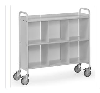
Modular system: bolted, tubular steel construction, powder coated light grey RAL 7035. Shelves and panels made of derived material timber board, pale grey. With 2 separating plates and longitudinal wall (back wall).4 swivel castors with TPE tyres, hubs with roller bearings. 2 swivel castors with wheel locks, according to the European Standard EN 1757-3 (safety of platform trolleys). Flat packed for easy self assembly.
