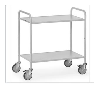
Modular system: bolted, tubular steel construction, powder coated light grey RAL 7035. 2 shelves of derived material timber board, pale grey. 4 swivel castors with TPE tyres, hubs with roller bearings. 2 swivel castors with wheel locks, according to the European Standard EN 1757-3 (safety of platform trolleys). Flat packed for easy self assembly.
