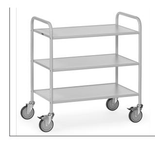
Modular system: bolted, tubular steel construction, powder coated light grey RAL 7035. 3 shelves of derived material timber board, pale grey. 4 swivel castors with TPE tyres, hubs with roller bearings. 2 swivel castors with wheel locks, according to the European Standard EN 1757-3 (safety of platform trolleys). Flat packed for easy self assembly.
