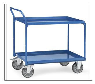
Modular system: Steel construction, welded. Tubular steel hoop and steel plate trays screwed. Trays oil-tight, rim 40 mm high, powder coated blue RAL 5007. 2 swivel and 2 fixed-wheel castors, TPE tyres, hubs with groove ball bearing. Swivel castors with wheel locks, according to the European Standard EN 1757-3 (safety of platform trolleys). Capacity of upper shelf 200 kg.
