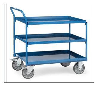
Modular system: Steel construction, welded. Tubular steel hoop and steel plate trays screwed. Trays oil-tight, rim 40 mm high, powder coated blue RAL 5007. 2 swivel and 2 fixed-wheel castors, TPE tyres, hubs with groove ball bearing. Swivel castors with wheel locks, according to the European Standard EN 1757-3 (safety of platform trolleys). Capacity of upper and middle shelf 200 kg.
