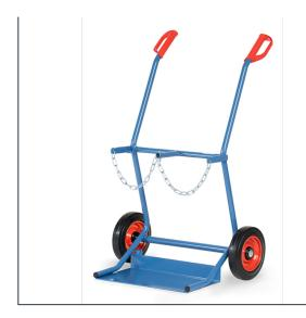
Welded and powder coated blue RAL 5007, tubular steel design. Bottle support with safety chain. Wheels with solid rubber tyres, hubs with roller bearings. For 2 bottles, each 20 litres contents, Ø 204 mm.
