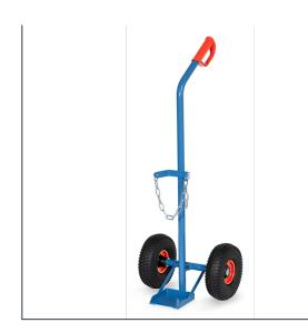
Welded and powder coated blue RAL 5007, tubular steel design. Bottle support with safety chain. Wheels with pneumatic tyres, hubs with roller bearings. For 1 steel bottle 10 litres content, Ø 140 mm.
