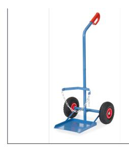
Welded and powder coated blue RAL 5007, tubular steel design. Bottle support with safety chain. Wheels with pneumatic tyres, hubs with roller bearings. For 1 propane gas bottle 11 kg  $\varnothing$  300 mm or 33 kg  $\varnothing$  318 mm.
