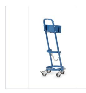
For 1 propane gas bottle 11 kg contents,  $\emptyset$  300 mm. Welded steel construction, powder coated blue RAL 5007. Interior- $\emptyset$  310 mm. With hose and shrink gun holder. 4 castor wheels, 2 with wheel locks. Solid rubber tyres 75 x 25 mm, hubs with ball bearings.
