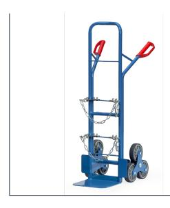
For transport on stairs. For 1 steel bottle of 20, 40 and 50 litres contents or 1 propane gas bottle 11 and 33 kg. Stairway truck TK 1325 is the basis product, additionally equipped with 4 perforated wide cross struts to screw bottle support with safety chain. With 2 three-armed wheel spiders, each equipped with 3 TPE tyres 160 mm Ø. Curved top bar and transversal struts. For safe transport of circular items such as rolls, cans, buckets etc.
