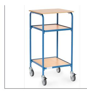
Steel tube and sectional steel welded, bolted construction, powder coated blue RAL 5007. Surface made of derived timber material 605 mm wide und 589 mm deep, with milled pen rest. 2 screw-down shelves, upper shelf centred shrewable for the possiility of 2 folders on top of each other. Capacity per shelf 50 kg. 4 swivel castors with TPE tyres 125 x 32 mm, 2 swivel castors with wheel locks, hubs with plain bearings. Easy movement across angles and barriers because of the big wheels.
