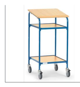
Steel tube and sectional steel welded, bolted construction, powder coated blue RAL 5007. Surface made of derived timber material, 605 mm wide und 590 mm deep, with stop bar. 2 screw-down shelves, upper shelf centred shrewable for the possiility of 2 folders on top of each other. Capacity per shelf 50 kg. 4 swivel castors with TPE tyres 125 x 32 mm, 2 swivel castors with wheel locks, hubs with plain bearings. Easy movement across angles and barriers because of the big wheels.
