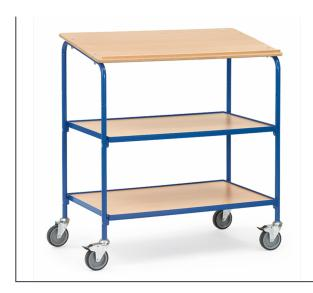
Steel tube and sectional steel welded, bolted construction, powder coated blue RAL 5007. Surface made of derived timber material, 1100 mm wide und 590 mm deep, with stop bar. 2 screw-down shelves, upper shelf centred shrewable for the possiility of 2 folders on top of each other. Capacity per shelf 50 kg. 4 swivel castors with TPE tyres 125 x 32 mm, 2 swivel castors with wheel locks, hubs with plain bearings. Easy movement across angles and barriers because of the big wheels.
