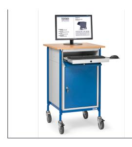
Steel tube and sectional steel welded, bolted construction, powder coated blue RAL 5007. With 1 lockable keyboard drawer with full extension and pull-out mouse pad. Horizontal writing desk, with cable slots in desktop and cupboard. Delivery without decoration. 4 swivel castors with TPE tyres 125 x 32 mm, 2 swivel castors with wheel locks, hubs with plain bearings. Easy movement across angles and barriers because of the big wheels.
