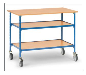
Steel tube and sectional steel welded, bolted construction, powder coated blue RAL 5007. Table board made of beech plywood, 20 mm thick, surface out of beech decoration. 2 screw-down shelves, variable distance of 50 mm, 1 x folder height possible. 4 swivel castors with TPE tyres 125 x 32 mm, 2 swivel castors with wheel locks, hubs with plain bearings. Capacity per shelf 50 kg. Table height 910 mm. Screw-down shelves 300 und 670 mm high, variable distance of 50 mm.
