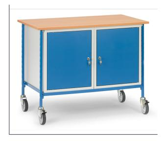
Steel tube and sectional steel welded, bolted construction, powder coated blue RAL 5007. Table board made of beech plywood, 20 mm thick, surface out of beech decoration. 2 lockable steel cupboards. Capacity per shelf in cupboards 30 kg. 4 swivel castors with TPE tyres 125 x 32 mm, 2 swivel castors with wheel locks, hubs with plain bearings. Capacity per shelf 50 kg. Table height 910 mm. Screw-down shelves 300 und 670 mm high, variable distance of 50 mm.
