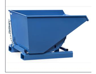
Self-tilting boxes need not to be lifted for emptying. The empty box moves automatically back into loading position. Sturdy welded 3 mm sheet steel design, powder coated in RAL 5007 blue. Standard-fitted fork-lift sleeves, anti-roll safety device and tilt lock. Link chain as anti-skidding and safety device. Traction cable to activate tilting mechanism, operated from fork-lift truck driver's seat.
