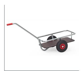
Light hand cart made of tubular steel, welded and galvanised. Suitable for outdoor area. Shaft can be screwed on. Platform made of water-resistant plywood boards. Wheels with pneumatic tyres. Hubs with roller bearings. Flat packed for easy self assembly.
