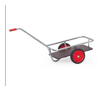
Light hand cart made of tubular steel, welded and galvanised. Suitable for outdoor area. Shaft can be screwed on. Platform made of water-resistant plywood boards. Wheels with solid rubber tyres. Hubs with roller bearings. Flat packed for easy self assembly.
