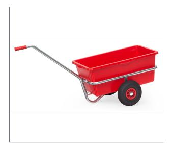
Light hand cart made of tubular steel, welded and galvanised. Suitable for outdoor area. Shaft can be screwed on. With Red plastic tray. Tray 90 liters content, L x W x H =  $715 \times 420 \times 320$  mm. Wheels with pneumatic tyres. Hubs with roller bearings. Flat packed for easy self assembly.
