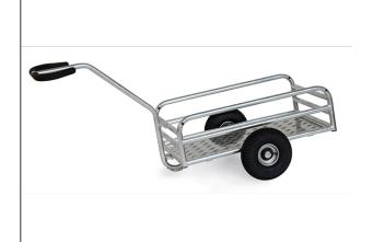
Handcart for use in outdoor areas. Welded from tubular steel, hot-dip galvanized. Platform made of quintet pattern aluminium plate. Rail 180/250 mm high with strong pipe struts. Shaft can be screwed on, with safety handle and skin-friendly soft grip cover. Large wheels with fibreglass-reinforced plastic wheel rim, with pneumatic tyres, hubs with roller bearings. Screwed wheel attachment for easy wheel change.
