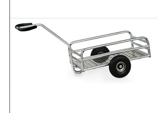
Handcart for use in outdoor areas. Welded from tubular steel, hot-dip galvanized. Platform made of quintet pattern aluminium plate. Rail 180/250 mm high with strong pipe struts. Shaft can be screwed on, with safety handle and skin-friendly soft grip cover. Large wheels with fibreglass-reinforced plastic wheel rim, with puncture-proof polyurethane tyres, hubs with roller bearings. Screwed wheel attachment for easy wheel change.
