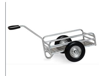
Handcart for use in outdoor areas. Welded from tubular steel, hot-dip galvanized. Platform made of quintet pattern aluminium plate. Rail 180/250 mm high with strong pipe struts. Shaft can be screwed on, with safety handle and skin-friendly soft grip cover. Large wheels with fibreglass-reinforced plastic wheel rim, with puncture-proof polyurethane tyres, hubs with roller bearings. Screwed wheel attachment for easy wheel change.
