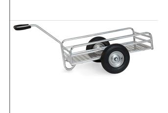
Handcart for use in outdoor areas. Welded from tubular steel, hot-dip galvanized. Platform made of quintet pattern aluminium plate. Rail 180/250 mm high with strong pipe struts. Shaft can be screwed on, with safety handle and skin-friendly soft grip cover. Large wheels with fibreglass-reinforced plastic wheel rim, with pneumatic tyres, hubs with roller bearings. Screwed wheel attachment for easy wheel change.
