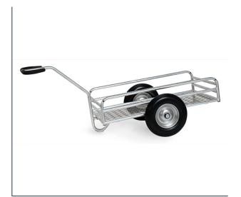
Handcart for use in outdoor areas. Welded from tubular steel, hot-dip galvanized. Platform made of quintet pattern aluminium plate. Rail 180/250 mm high with strong pipe struts. Shaft can be screwed on, with safety handle and skin-friendly soft grip cover. Large wheels with fibreglass-reinforced plastic wheel rim, with puncture-proof polyurethane tyres, hubs with roller bearings. Screwed wheel attachment for easy wheel change.
