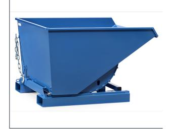
Self-tilting boxes need not to be lifted for emptying. The empty box moves automatically back into loading position. Sturdy welded 3 mm sheet steel design, powder coated in RAL 5007 blue. Standard-fitted fork-lift sleeves, anti-roll safety device and tilt lock. Link chain as anti-skidding and safety device. Traction cable to activate tilting mechanism, operated from fork-lift truck driver's seat. Item number with addition "A" means "with drainage tap".
