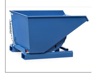
Self-tilting boxes need not to be lifted for emptying. The empty box moves automatically back into loading position. Sturdy welded 3 mm sheet steel design, powder coated in RAL 5007 blue. Standard-fitted fork-lift sleeves, anti-roll safety device and tilt lock. Link chain as anti-skidding and safety device. Traction cable to activate tilting mechanism, operated from fork-lift truck driver's seat. Item number with addition "A" means "with drainage tap".
