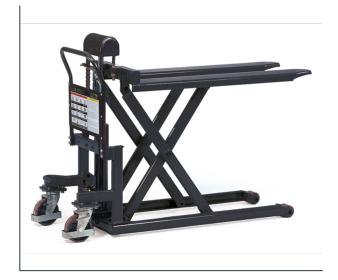
Excellent stability under load and travelling even with lifted load. Frame and forks made in sectional steel construction, powder coated, anthracite grey RAL 7016. Sturdy tubular push handle. Hydraulic pump with chromium-plated piston and overload valve. Operated via pedal control. Lowering valve to be operated via hand lever. 2 castor wheels with
