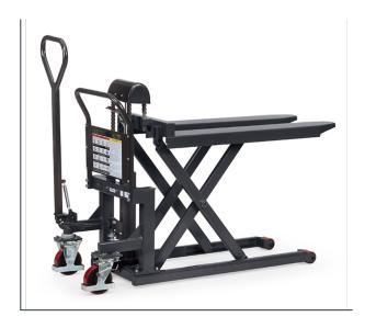
Excellent stability under load and travelling even with lifted load. Frame and forks made in sectional steel construction, powder coated, anthracite grey RAL 7016. Sturdy tubular push handle. Hydraulic pump with chromium-plated piston and overload valve. Operated via pedal control. Lowering valve to be operated via hand lever. 2 castor wheels with lock. Version is additionally equipped with a steering shaft.
