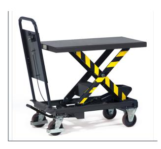
Sectional steel/steel plate construction, powder coated anthracite RAL 7016. Sturdy tubular push handle. Hydraulic pump with chromium-plated piston. Operation via pedal control. Lowering valve precisely adjustable via hand lever. 2 castor and 2 fixed wheels, wheels with Polyurethanee tyres, castor wheels with lock. Tubular push handle fixed with screws.
