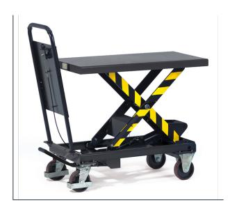
Sectional steel/steel plate construction, powder coated anthracite RAL 7016. Sturdy tubular push handle. Hydraulic pump with chromium-plated piston. Operation via pedal control. Lowering valve precisely adjustable via hand lever. 2 castor and 2 fixed wheels, wheels with Polyurethanee tyres, castor wheels with lock. Tubular push handle fixed with screws.
