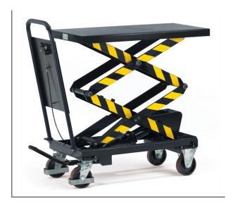
Sectional steel/steel plate construction, powder coated anthracite RAL 7016. Sturdy tubular push handle. Hydraulic pump with chromium-plated piston. Operation via pedal control. Lowering valve precisely adjustable via hand lever. 2 castor and 2 fixed wheels, wheels with Polyurethanee tyres, castor wheels with lock. Double shears for enlarged lifting range. Tubular push handle fixed with screws.
