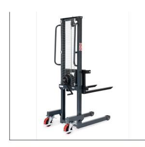
For the occasional use as lifting and transport appliance. Sturdy sectional steel construction with tubular push handles, powder coated anthracite RAL 7016. Maintenance free. Lifting by means of safety hand winch. Forks adjustable. 2 castor wheels, wheels with Polyurethanee tyres 150 x 40 mm and 2 fork rollers nylon 80 x 47 mm. Castor wheels with lock. Load center distance: 400 mm, stroke per crank turning: 40 mm, total height 2030 mm.
