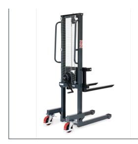
For the occasional use as lifting and transport appliance. Sturdy sectional steel construction with tubular push handles, powder coated anthracite RAL 7016. Maintenance free. Lifting by means of safety hand winch. Forks adjustable. 2 castor wheels, wheels with Polyurethanee tyres 150 x 40 mm and 2 fork rollers nylon 80 x 47 mm. Castor wheels with lock. Load center distance: 400 mm, stroke per crank turning: 40 mm, total height 2030 mm.
