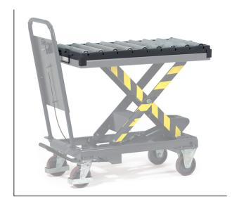
Sectional steel frame with holding angles and 2 upward tilting stops, powder coated anthracite RAL 7016. 9 steel rolls (Ø 57 mm and length 430 mm) with roller bearings. Distance between axles 112,5 mm, height 64 mm, carrying capacity 500 kg - rigid-
