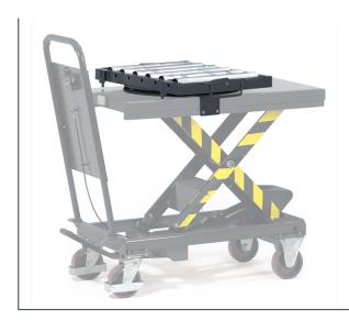
Can be fixed to platform with clamped joint, swivelling by 360Ű, arrestable. 6 steel rolls (Ã? 57 mm and length 430 mm) with roller bearings. Distance between axles: 110 mm Height 92 mm, carrying capacity 500 kg - swivelling -
