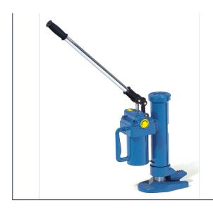
For lifting of machines and other heavy loads. Easy lifting with lifting claw and end plate by means of installed hydraulic hand pump. Precise lowering via lowering valve, overload valve. Pump lever detachable. Swivelling of housing by 360°, variable range of application. Sturdy compact steel construction, coating blue RAL 5007.
