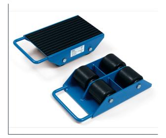
For the easy and safe transport of heavy goods such as containers, boxes, machines etc. Sturdy welded steel construction with handles made of round or tubular steel, powder coated blue RAL 5007. Carrying platforms with anti-slip rubber cover. Big nylon rolls with roller bearings. High carrying capacity combined with low net weight. Outside dimensions L x W x H: 400 x 228 x 100 mm. Scope of delivery: 1 piece
