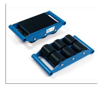
For the easy and safe transport of heavy goods such as containers, boxes, machines etc. Sturdy welded steel construction with handles made of round or tubular steel, powder coated blue RAL 5007. Carrying platforms with anti-slip rubber cover. Big nylon rolls with roller bearings. High carrying capacity combined with low net weight. Outside dimensions L x W x H: 415 x 210 x 100 mm. Scope of delivery: 1 piece
