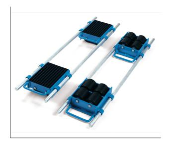
Moving gear for the easy and safe transport of machines and other heavy goods. Sturdy welded steel construction with handles made of round steel, powder coated blue RAL 5007. Carrying platforms with anti-slip rubber cover. Big nylon rolls with roller bearings. Scope of delivery: 2 transport rollers and 2 connecting rods made of round steel. Warranty: 2 years.
