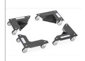
For moving of furniture or similar box-shaped objects. Low loading edge and safe transport. Steel plate housing welded, coated signal red, loading platform with non-slip covering. 3 solid rubber castors 50 x 20 mm. Scope of delivery: 1 set = 4 pieces (in a plastic box)
