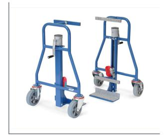
Manual crank for one man transport of cupboards, lockers etc. Steel tubular construction, powder coated blue RAL 5007. Winch with manual crank arm. Crank protected by a C-profile. Adjustable supports with protective covering. Loading surface with anti-slip covering. Two steering wheels with non-marking Polyurethanee tyres and non-tracking elasticated solid rubber tyres, hub with roller bearings. One fixed 5 m long strap. Delivered in pairs.
