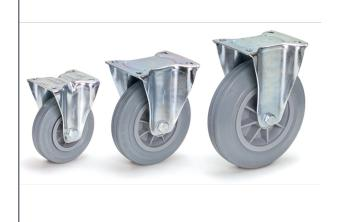
Casings made of steel sheet, galvanized. Wheels with blue-grey solid rubber tyres, non-marking (trackless), plastic rims, hubs with roller bearings.
